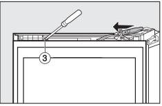
Attach the spacer and the soft-close mechanism securely using screw 3.
